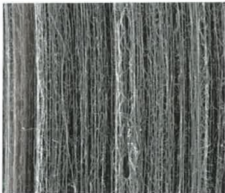
▲ Figure 2-10 Carbon nanotubes (CNT). A tubular form of carbon, with a diameter as small as 1 nm, is produced from sheets rolled into tubes. (NASA Ames)
