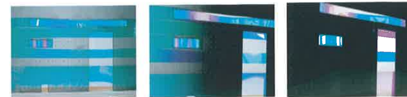
▲ Figure 1-6 Design experiment: view directional film and radiant color film have been used together in this façade study. (Nyriabu Nyriabu)
