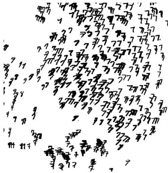
MNIST dataset mapped to a 2D space based on similarities (t-SNE algorithm) shows different styles of handwritten 7 ( https://lvdmaaten.github.io/tsne/ )
